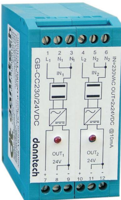
The Coupling Card or Digital Input Converter is designed to provide an isolated DC output suitable for a PLC input from a 115 or 230 VAC signal.
